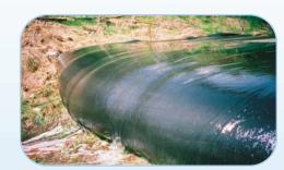
Clear effluent flows from a Geotube® unit. In many cases, filtrate is directly discharged with no additional treatment.
